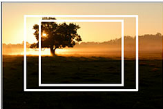
The three most common sensor sizes compared: full frame, APS-C and Four-thirds. Smaller sensors 'crop' the scene and make a lens appear to have a longer focal length.
